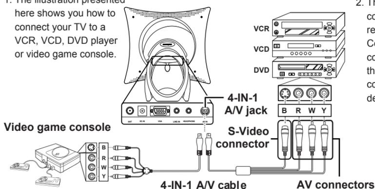
2. The cables are color-coded (black, red, white, and yellow). Connect each color-coded cable to the appropriate connector on your device.
