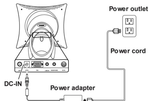
1. Connect the power cord to the power adapter as illustrated.
