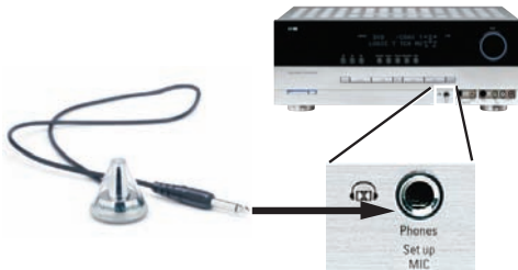
Figure 46 – Plug EzSet/EQ microphone into receiver.
