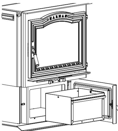
opening the ash door and removing the ash pan, open the bypass damper. Wearing heavy protective gloves, open the ash door and remove the ash pan by pulling it forward by the handle. Close the ash door and damper bypass before taking the ashes outside for safe disposal.
