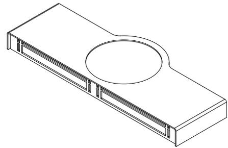
The top air grill installs over the flue collar and simply rests on the top of the stove. The brushed stainless grill is included with this option as well.
