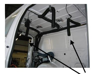
Attach the "Y" duct hose adaptor to the 8 foot front duct hose and connect both 4 foot hoses from "Y" to vents in driver and passenger side front ceiling. This will provide a total of four ceiling vents.
