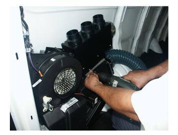
There are two (2) ducts on the factory HVAC unit. One at rear is for air conditioning and one forward is for heat. The 4" blue hose connects heat into the new plenum.
