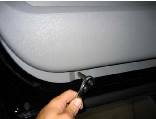
Remove hex head screws holding lower section of door panel
