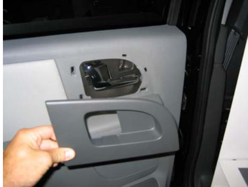
Remove plastic trim piece. Metal clips hold on trim
