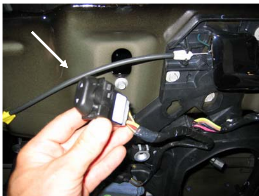
Remove window switch and reconnect. Wire tie switch in safe location.
