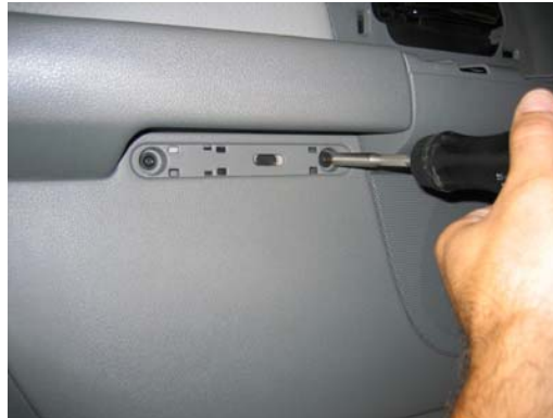
Remove trim piece covering torx screws under door panel armrest and remove screws
