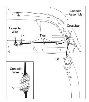
8. Set the console assembly on the brackets on the Left and Right Uprights (88, not shown). **Be careful not to pinch any wires.**
