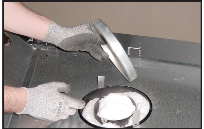
Figure 7.4 Remove the seal cap.
