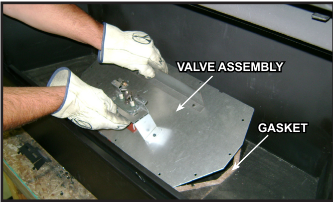
Figure 16.6 Remove Valve Plate
