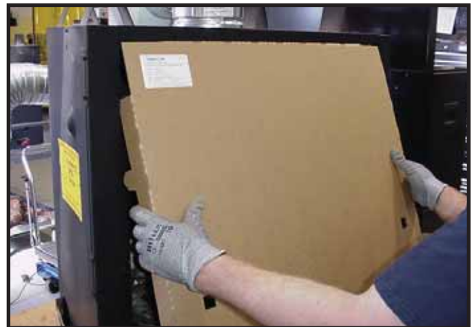
Figure 13.8 Installation of Splatter Guard
