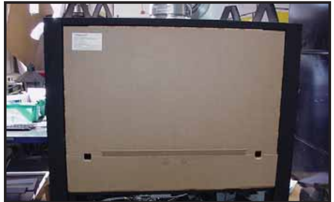
Figure 13.14 Splatter Guard with Lower Access Panel Open
