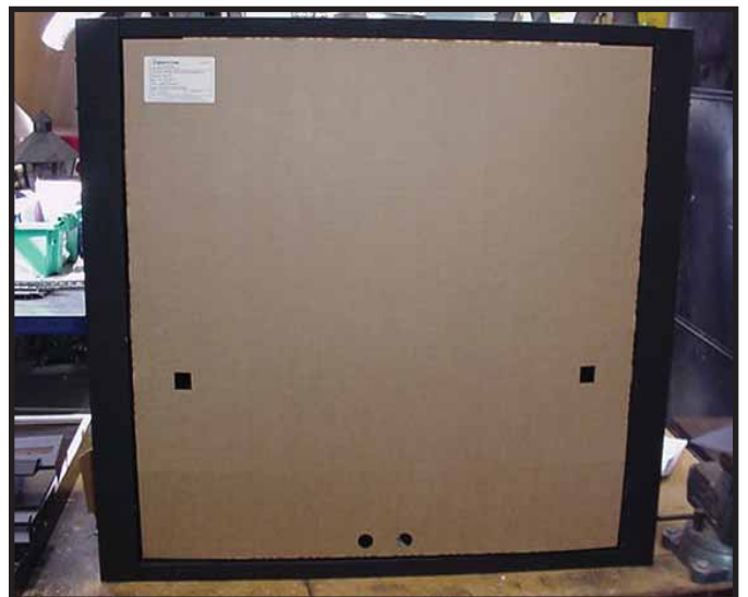
Figure 13.15 Splatter Guard with Lower Access Panel Closed
