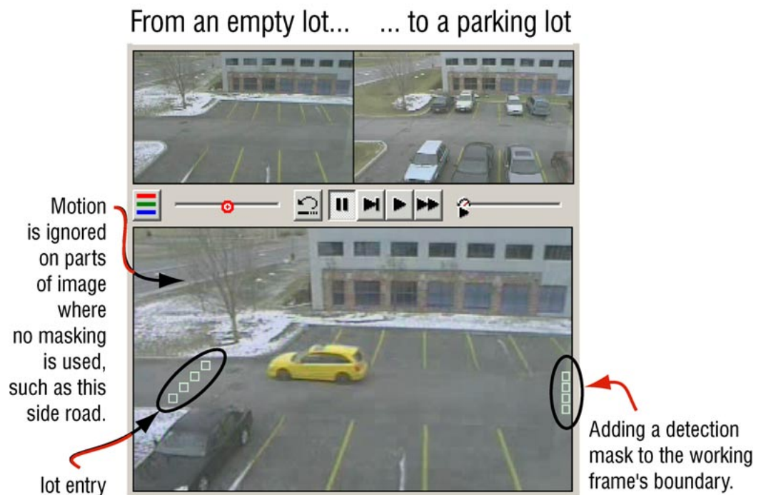
Fig. 53. Masking the entrance/exit to a parking lot. You can search for arrival and departure times by using masks at entry points to an area, and/or at the boundaries of an image. Use of a mask excludes unmasked areas from being searched for movement.
