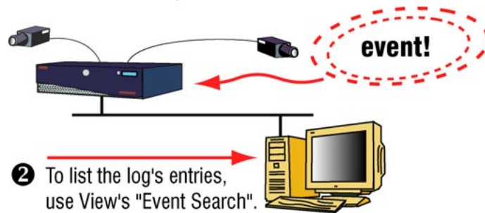
Fig. 76. You can set a Rapid Eye Multi-Media unit to log an event.
