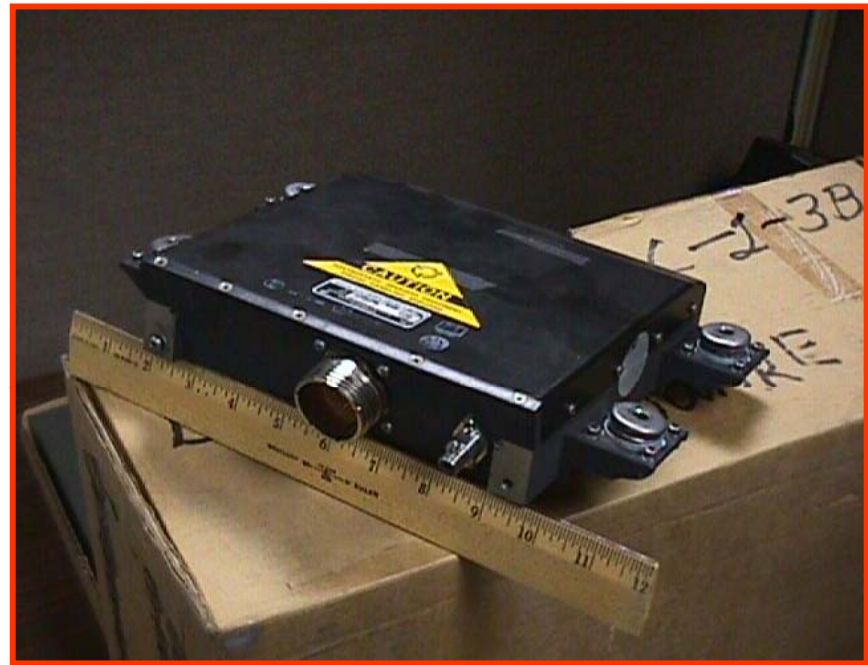
TFE731-20/40/50/60 DEEC (Production) - Engine mounted*- TFE731-50 DEEC in Hawker 900XP is fuselage mounted
