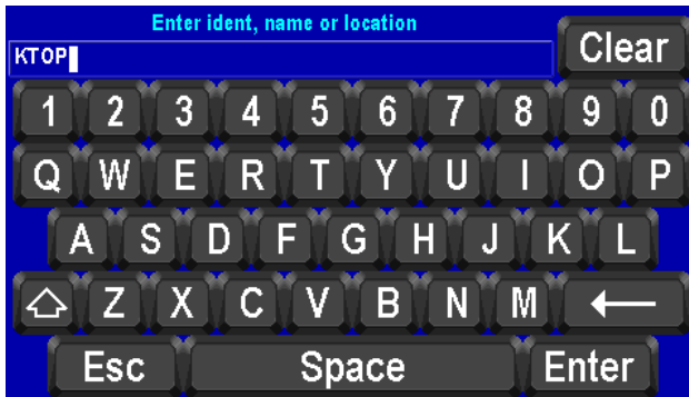
Figure 3-58: Enter Waypoint Identifier
