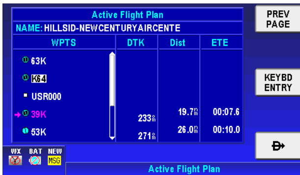
Figure 3-38: Bypass a WPT - Step 3
