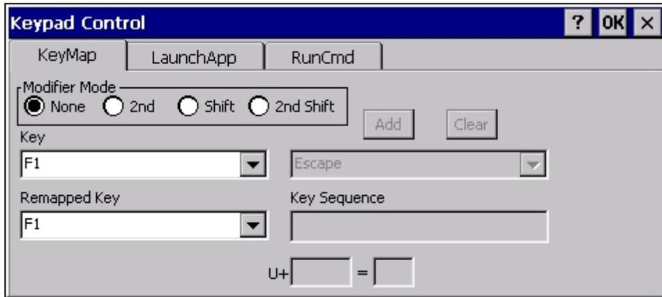
Assign settings by clicking radio buttons and selecting keys from the drop down boxes. Tap the OK button when finished. The changes take effect immediately.
