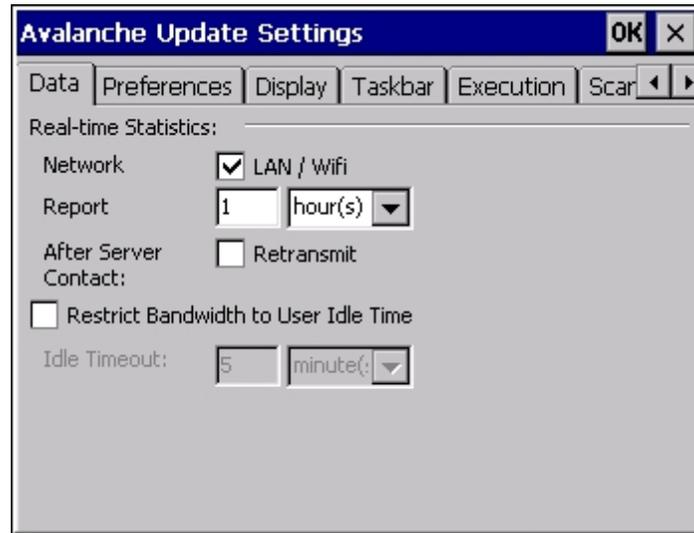
The Data tab controls when data is transferred between the MX3Plus and the Mobile Device Server.
