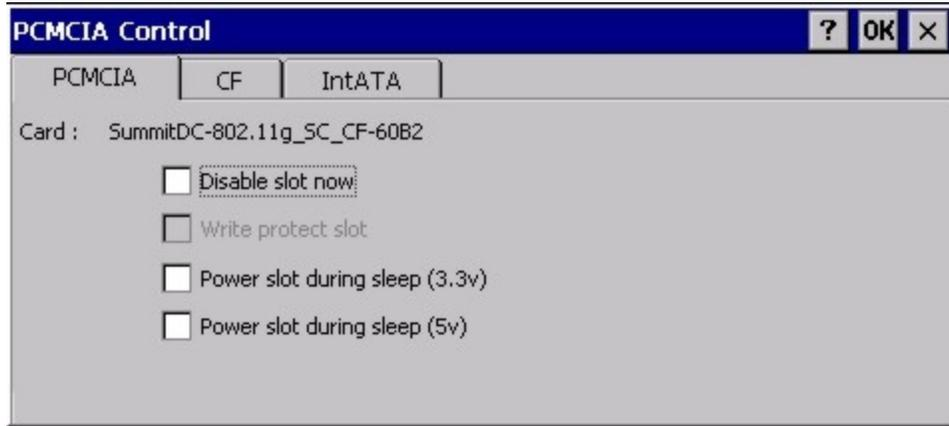
The name of the card (from the CIS data on the card) in the slot is displayed. This information cannot be changed by the user. When "Power slot during sleep" is checked, the slot will stay powered up in Suspend at the cost of reduced battery life. When "Disable slot now" is checked, the slot is powered down as soon as the Control Panel is closed and the PCMCIA driver ignores any card in the slot. When there is no card in a slot, the options are dimmed.
