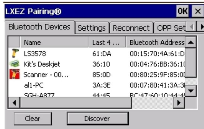
The discovered paired devices may or may not be identified with an icon. Discovered devices without an icon can be paired as a Scanner or a Printer. The Bluetooth panel assigns an icon to the device name.
