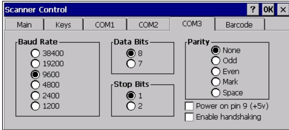
This panel sets communication parameters for any device connected to the external port.
