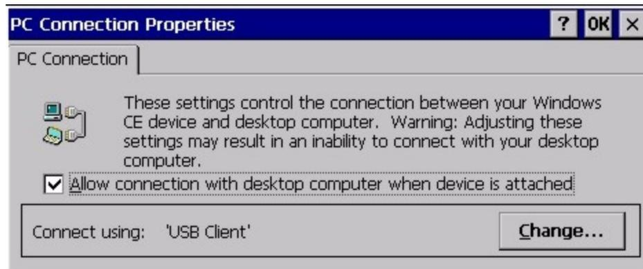
Unchecking the **Allow connection with desktop computer when device is attached** checkbox disables ActiveSync on the MX3Plus.
