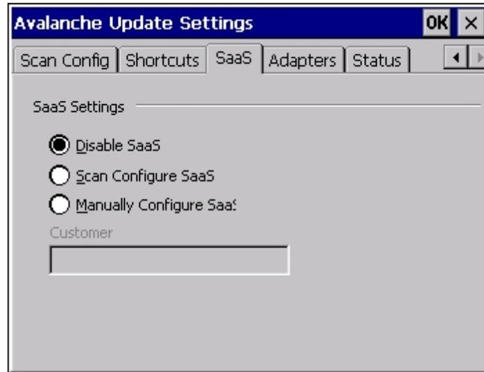
Use to configure the Enabler to connect with Avalanche on Demand. This is a Software-as-a-Service version of Avalanche. Using either of the SaaS configuration options below assumes the user has registered with Wavelink.
