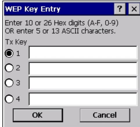
Valid keys are 10 hexadecimal or 5 ASCII characters (for 40-bit encryption) or 26 hexadecimal or 13 ASCII characters (for 128-bit encryption). Enter the key(s) and click **OK**.
