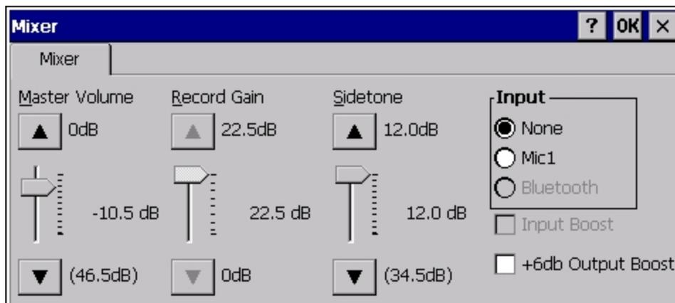
Select the input for the mixer. Move the sliders up and down, or tap the up and down arrows, to adjust the decibel level.
