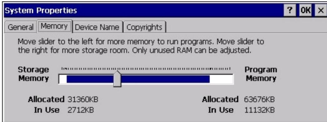
Move the slider to allocate more memory for programs or storage. If there isn't enough space for a file, increase the amount of storage memory. If the mobile device is running slowly, try increasing the amount of program memory.
