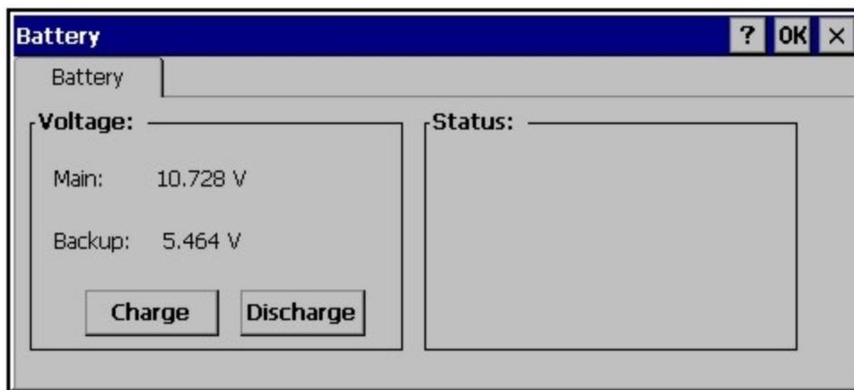
The backup battery draws power from the Main battery to maintain a charge. The backup battery voltage and percentage of power fluctuate continuously.
