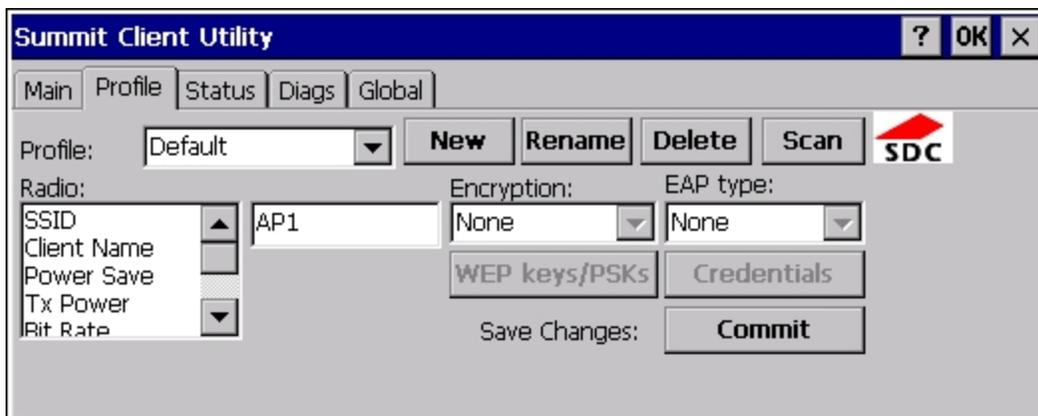
When logged in as an Admin (see [Admin Login](#)), use the Profile tab to manage profiles. When not logged in as an Admin, the parameters can be viewed, and cannot be changed. The buttons on this tab are dimmed if the user is not logged in as Admin. The Profile tab was previously labeled Config.
