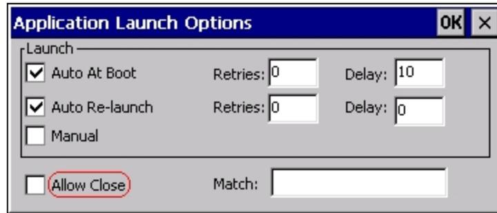
Default is Disabled. When enabled, the associated application can be closed by the end-user.
