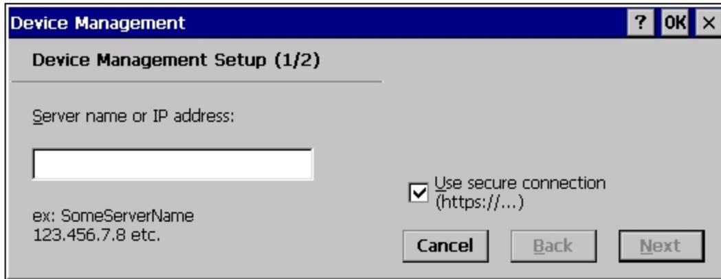
Specify the server name or IP address of management server and check the checkbox if a secure connection is to be used. Refer to the Microsoft.com website for more information on device management for Windows CE equipped devices.
