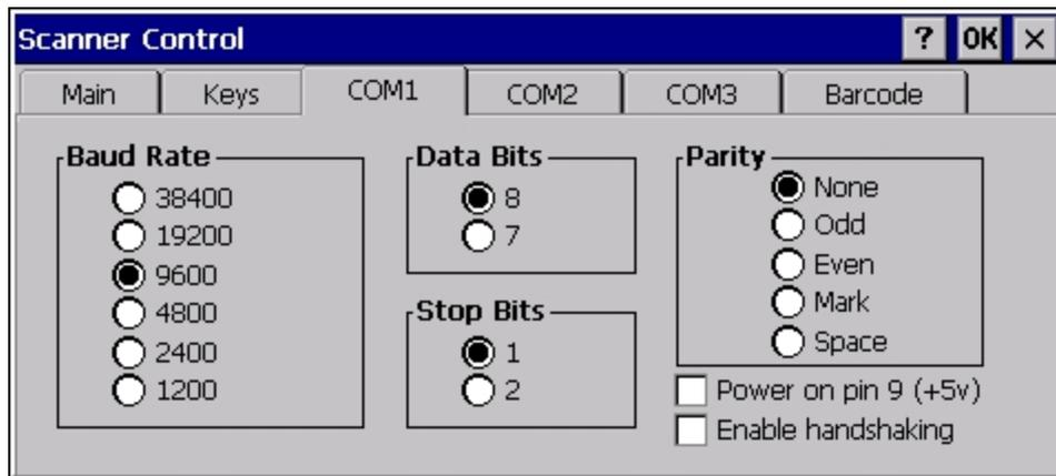
This panel sets communication parameters for any device connected to the external port. The settings for COM1 port on the MX3-RFID are pre-set and dimmed. Settings cannot be changed by the end-user. Baud rate is 115200, 8 data bits, 1 stop bit, no parity and power on Pin 9 is enabled.
