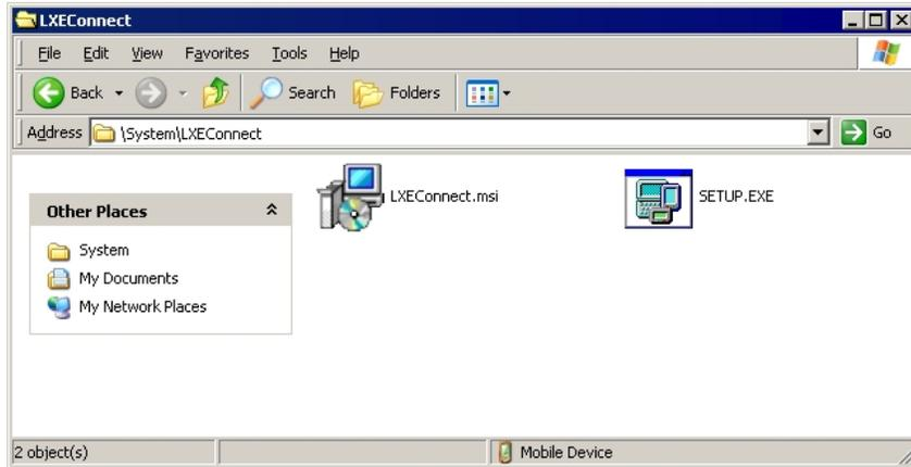
7. Select and copy the LXEConnect.msi and Setup.exe files from the MX3Plus to the user PC. Note the location chosen for files
