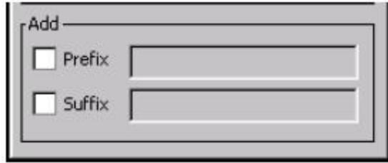
Use this option to specify a string of text, hex values or hat encoded values to be added to the beginning (prefix) or the end (suffix) of the bar code data. Up to 19 characters can be included in the string. The string can include any character from the keyboard plus characters specified by hex equivalent or entering in hat encoding. Please see *Hat Encoding and Decimal-Hexadecimal Chart* sections in the *Appendix* for a list of characters with their hex and hat-encoded values.
