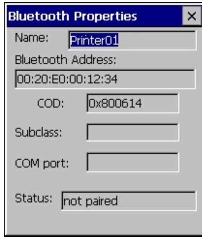
Data on the Bluetooth Properties panel cannot be changed by the user. The data displayed is the result of the device Query performed during the Discovery process.
