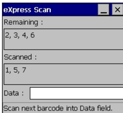
The remaining bar codes may be scanned in any order. After a bar code is scanned, that bar code is removed from the "Remaining:" list and placed in the "Scanned:" list.
