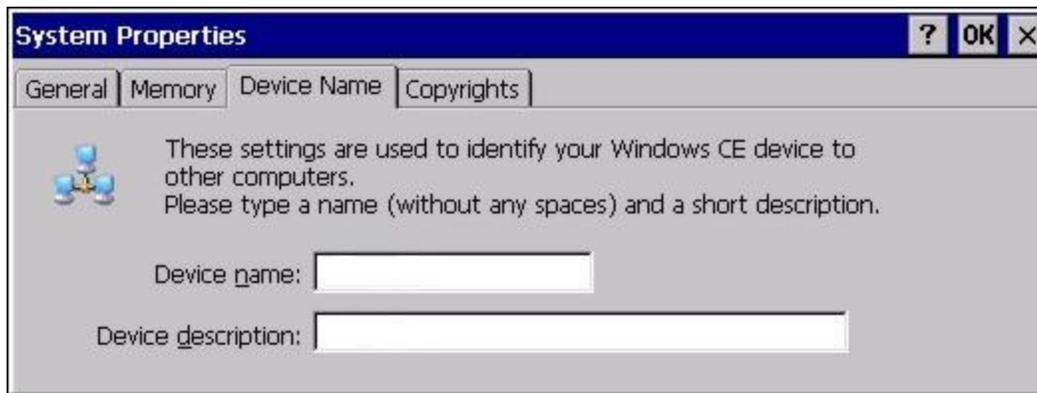
The device name and description can be changed by the user. Enter the name and description using either the keypad or the Input Panel and tap OK to save the changes. This information is used to identify the MX3Plus to other computers and devices.
