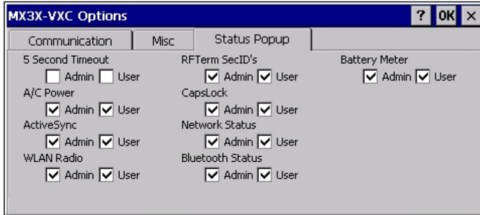
Using the [key mapping control panel](#), the System Administrator must first assign a **Status User** key sequence for the end-user when they want to toggle the Status Popup Window on or off.
