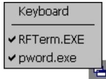
A checkmark on the switchpad menu indicates applications currently active or available for Launching by the user. When Keyboard is selected, the MX3Plus default input method (Input Panel, Transcriber, or custom input method) is activated.
