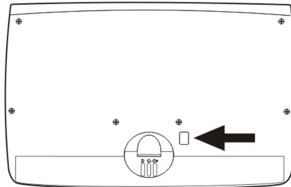
The IR operating envelope has a distance range of 2 cm (.79 inches) to 1 meter (3.2 feet) with a viewing angle of 30 degrees.
