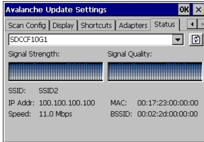
Link speed indicates the speed at which the signal is being sent from the adapter to the MX3Plus. Speed is dependent on signal strength.
