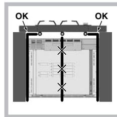
! If the appliance is fitted under the counter, make sure that the hob piping is positioned correctly and that it does not interfere with the oven during installation or obstruct the rear vents of the cooling fan.
