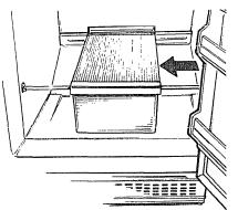
4. Place your hand on the drawer cover and pull the drawer out. Then lift the cover and remove it.
