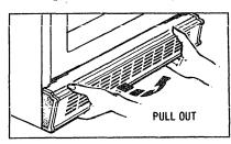
To adjust rollers or leveling legs, remove the base grille by grasping it at the bottom and pulling it out.
