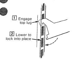
To replace shelves: Select desired shelf height. With shelf front raised slightly, engage top lugs in tracks at rear of cabinet. Then lower front of shelf until it locks into position.
