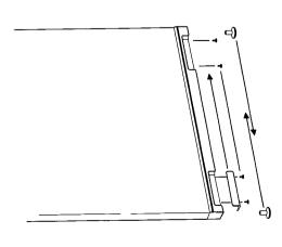
Refit the top door, sliding it upwards, locating the top hinge pin in the door hinge bush.
