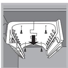
If you need more storage space, the ICE DEVICE may be taken out after you have removed the 4 fixing screws.
