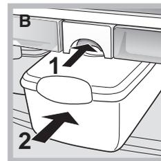
4. Press the button on the shelf and place the container in the central position (see figure B).
