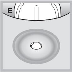
10. To open the container, turn the knob anticlockwise to the OPEN position (*see figure A*): this will allow air to enter the container and make it easy to open. The valve will move upwards as air enters the container (*see figure E*).
