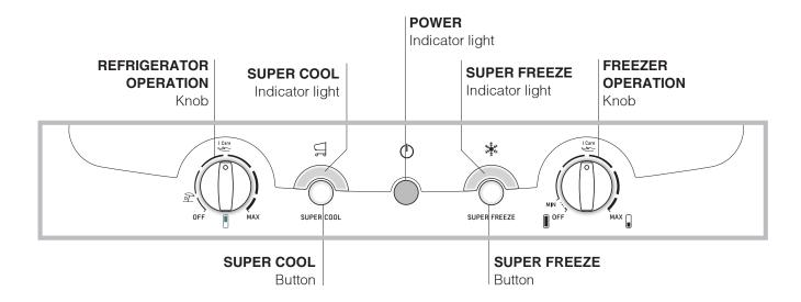
REFRIGERATOR OPERATION Knob to regulate the temperature of the refrigerator compartment.
