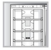
The No Frost system, thanks to the presence of a number of aeration cells, enables the constant circulation of air inside the compartment, while the internal temperature of the refrigerator is kept even using the same compartment ventilation system.
