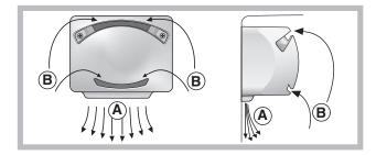
Pure Wind System maximises air circulation, improving the efficiency of the evaporator and helping to achieve the optimal temperature inside the refrigerator as quickly as possible each time it has been opened. The blown air (A) is cooled when it comes into contact with the cold wall, whereas the hotter air (B) is sucked up (see diagram).
