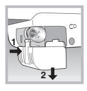
Access the light bulb by removing the cover as indicated in the diagram. Replace it with a similar light bulb within the power range indicated on the cover (max 10W).
