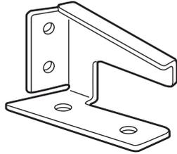
Fixed to the floor or wall at the rear of the fridge, the stability bracket hooks onto the compressor mounting plate holding the fridge secure.
