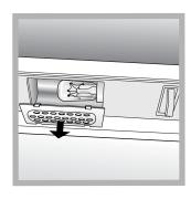
Access the light bulb by removing the cover as indicated in the diagram. Replace it with a similar light bulb within the power range indicated on the cover (10W).
