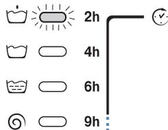
Once the set delay is complete, the flashing LED will turn off and the programme set will start.
