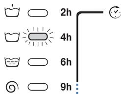
As time passes, the remaining delay will be displayed, and the corresponding LED will flash:
