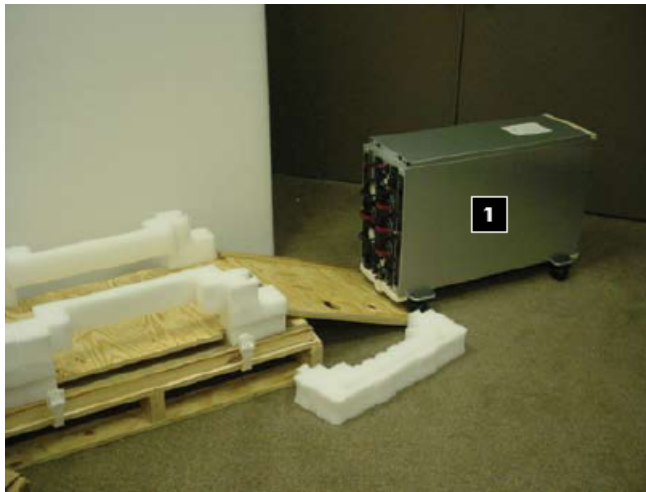
Figure 3-6 Rolling the Unit to the Installation Location
