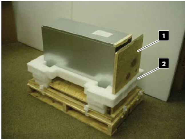
Figure 3-3 Removing the Ramp and Front Cushion
