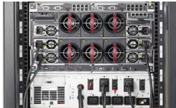
Figure 8. Redundant HP BladeSystem c3000 power supplies connected to an HP R5500 UPS
