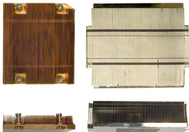
Figure 6. Processor heat sink using fully ducted design (left) and a traditional heat sink in a 1U rack-mount server (right)
