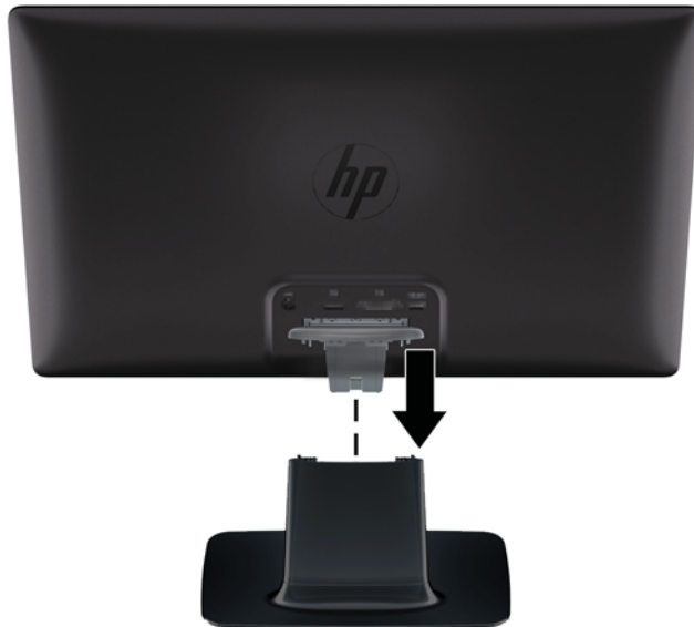
Figure 3-2 Inserting the Monitor Panel
