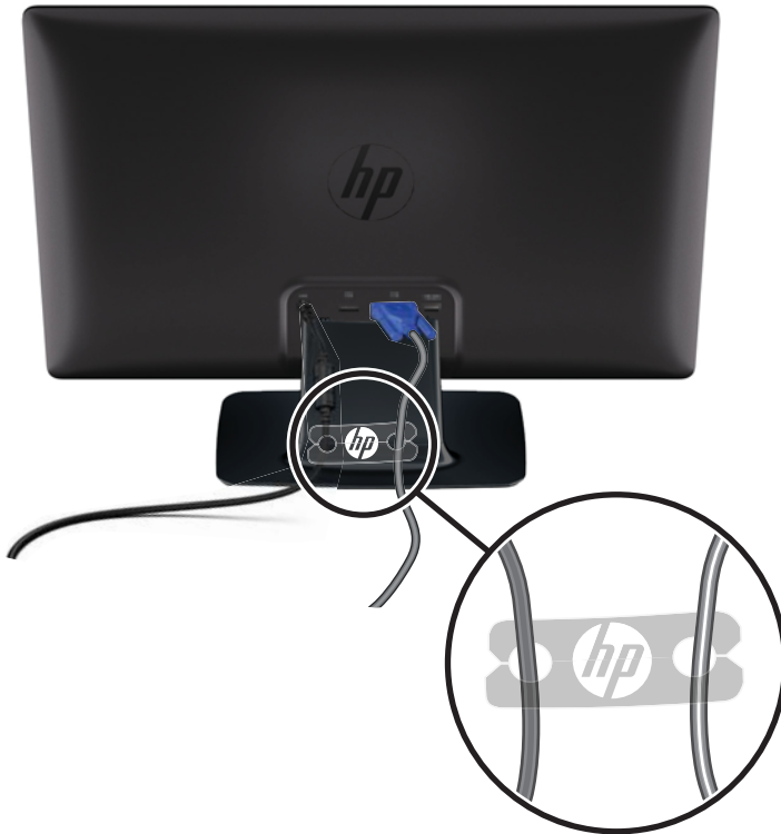
Figure 3-7 Installing the Cable management Clip
