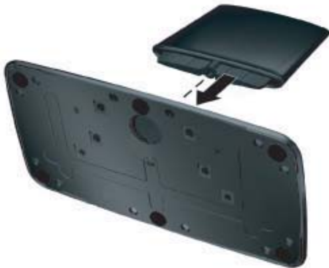
Figure 3-1 Assembling the Base and Pedestal
