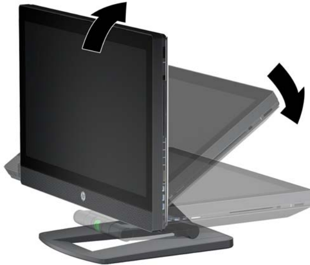
Figure 3-13 Maneuver workstation to horizontal position
