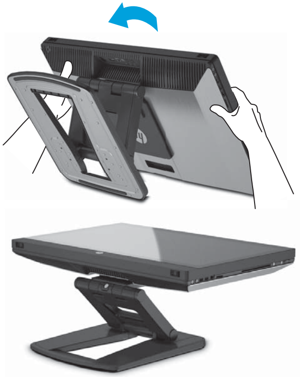
Figure 3-5 Tilt the unit towards you after connecting cables
