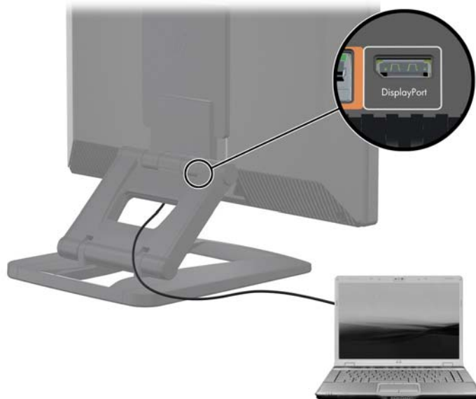
Figure 3-17 Connecting the display ports
