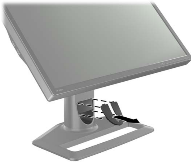
Figure 2-9 Cable Routing Cover
