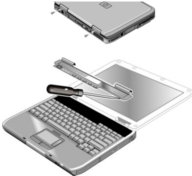
Figure 2-9. Removing the Keyboard Cover
