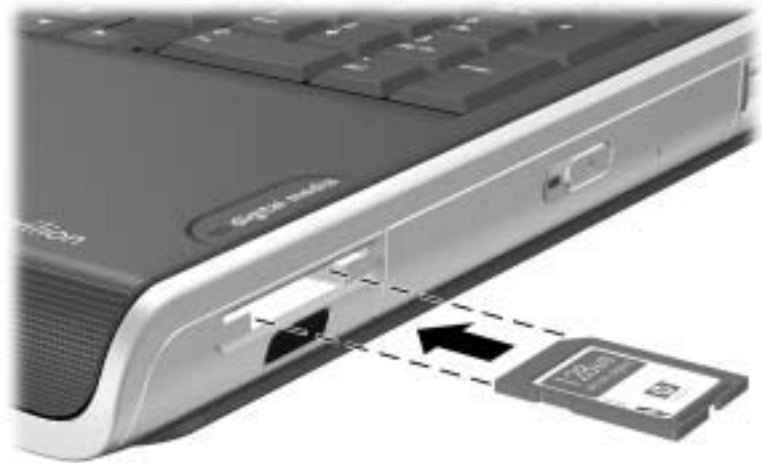
Inserting a digital media card
