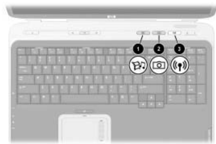
Identifying the Quick Launch buttons
