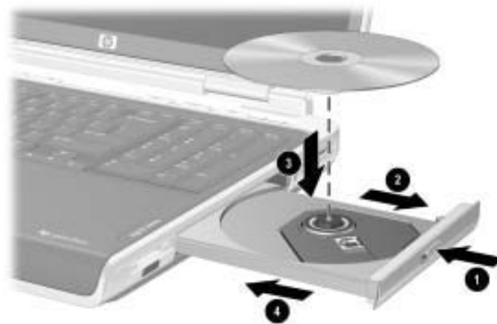
Inserting an optical disc into the optical drive
