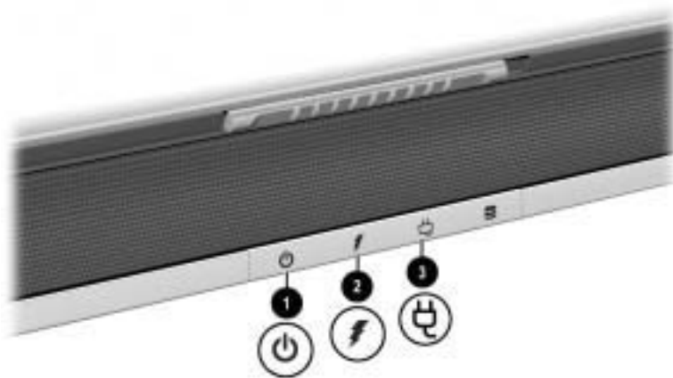
Identifying the battery and power/standby lights
