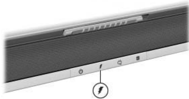
Identifying the battery light
