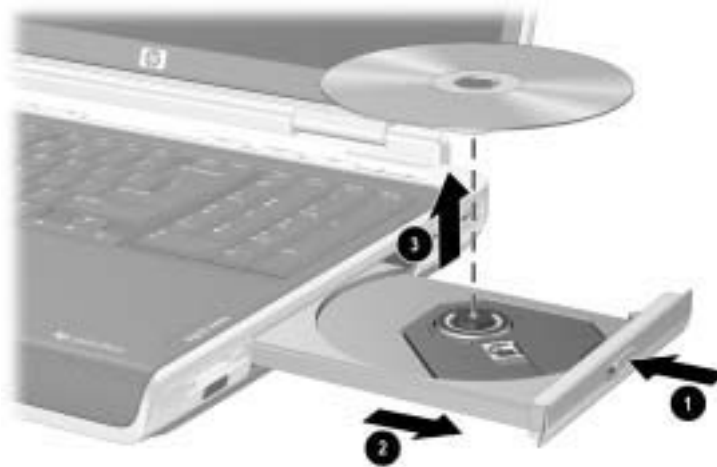
Removing an optical disc from the optical drive when power is available
