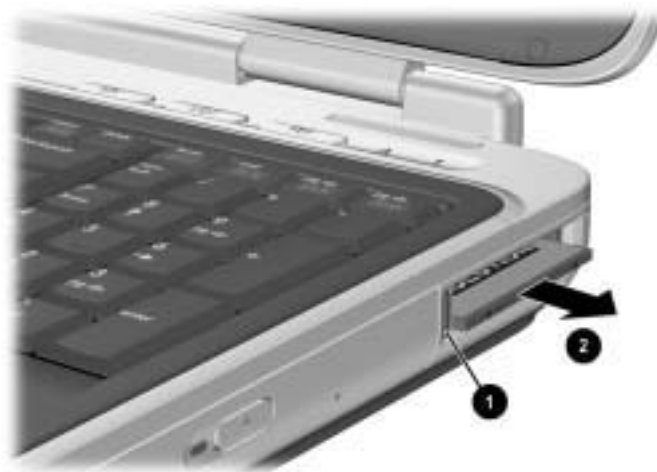
Removing a PC Card
