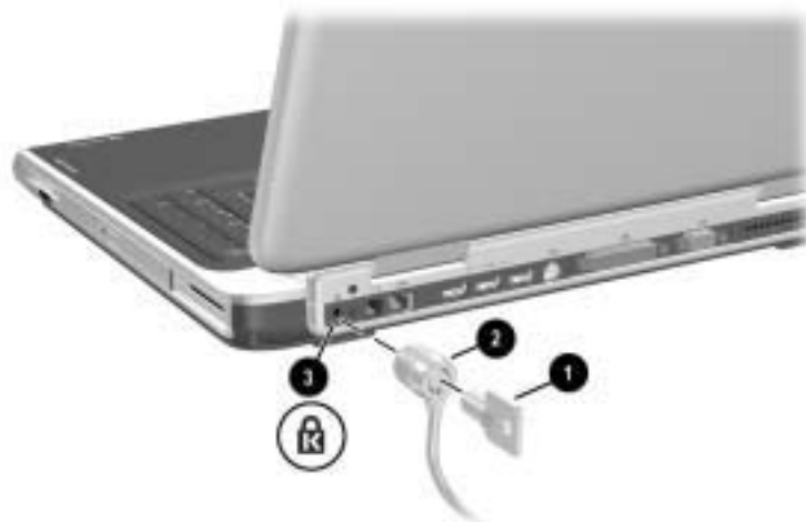
Connecting an optional cable lock
