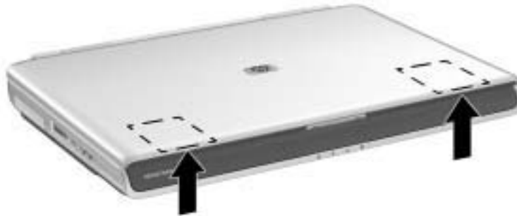
Wireless antennae location
