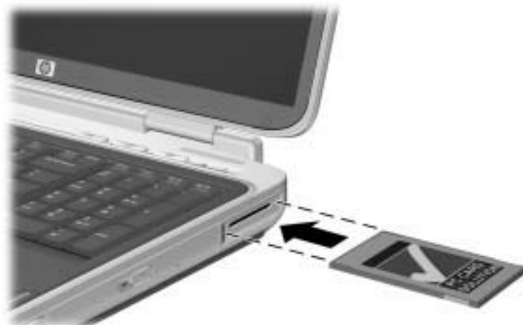
Inserting a PC Card
