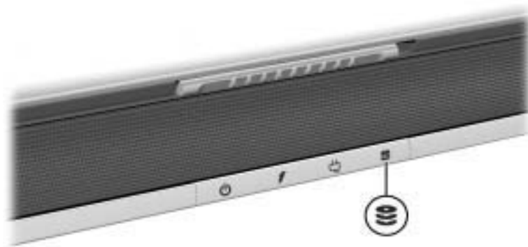
Identifying the hard drive activity light
