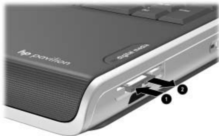
Releasing and removing a digital media card
