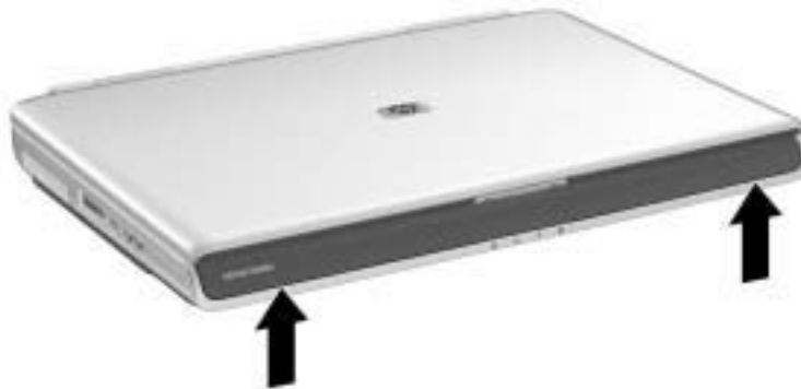
Identifying the internal speakers
