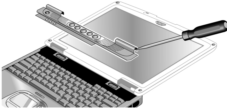
Figure 2-7. Removing the Keyboard Cover
