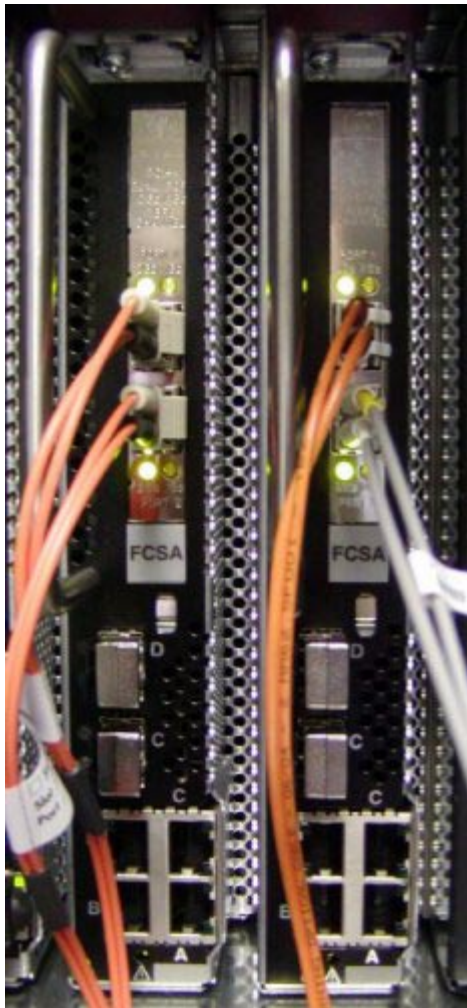
Figure 3-6. View of Two FCSAs at the Rear of Server
