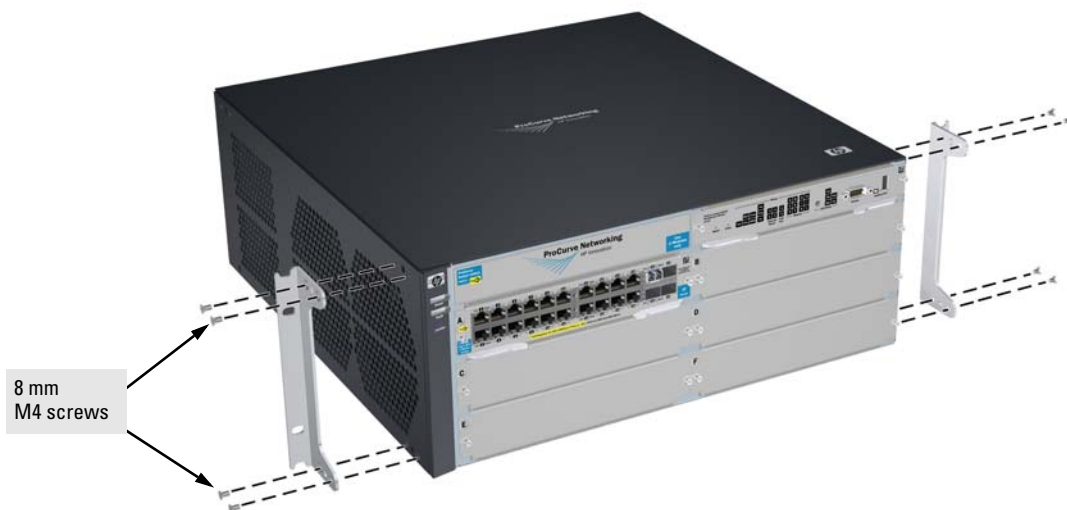
Figure 2-7. Attaching Brackets to the 5400zl Switch
