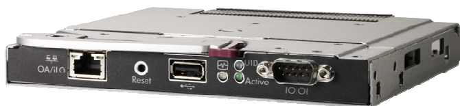
Figure 7. HP Onboard Administrator management module
