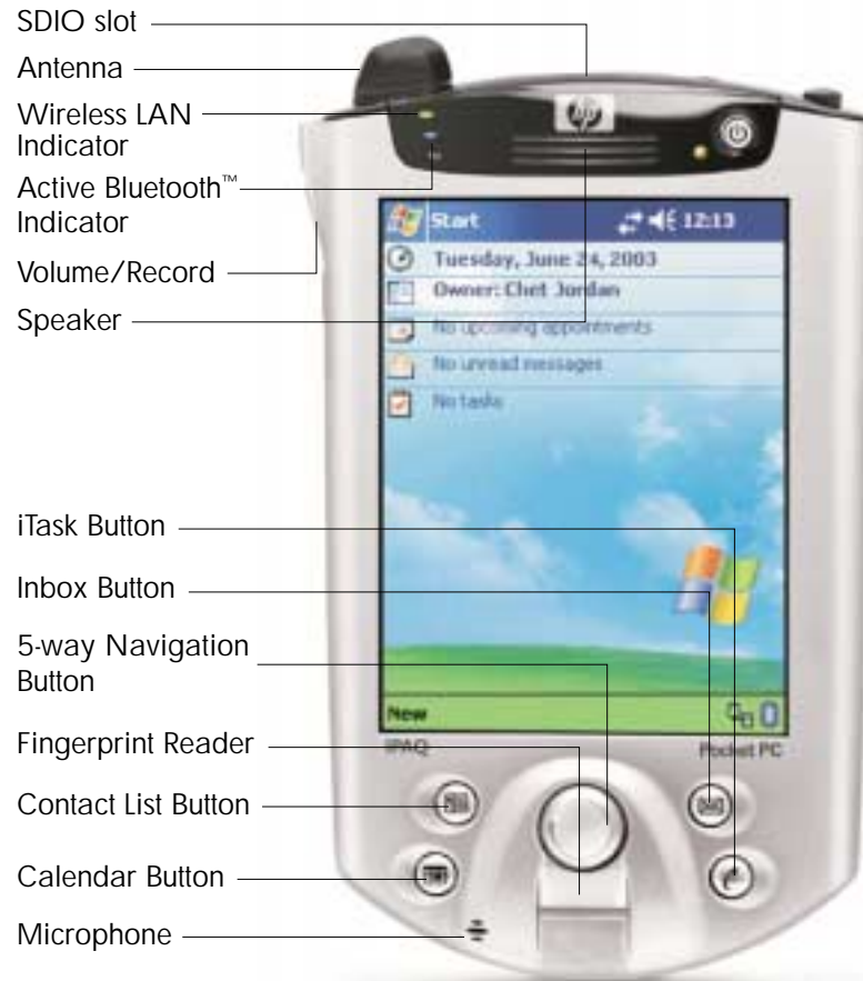
The HP iPAQ models in the h5500 series are Microsoft® Windows® Powered Pocket PCs
