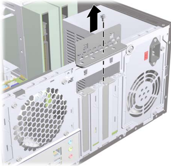
Figure 6-8 Opening the Slot Cover Lock
