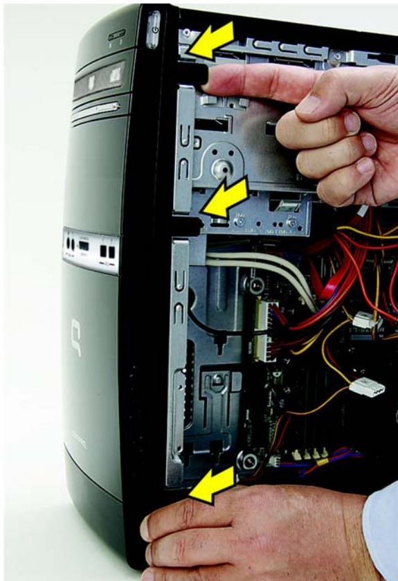
Figure 2-4 Removing the Front Bezel
