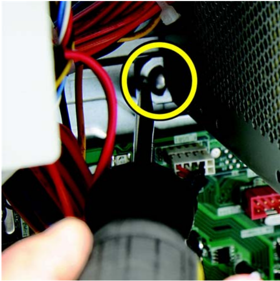
Figure 2-57 Pressing the power supply latch
