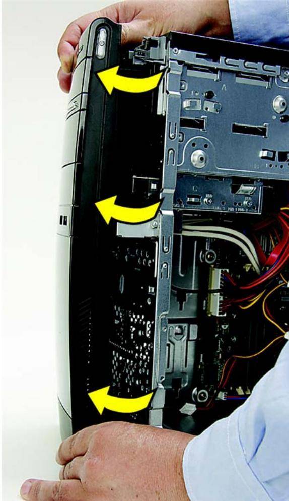
Figure 2-5 Removing the Front Bezel
