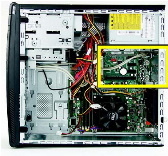
Figure 2-12 Locating the expansion card slots
