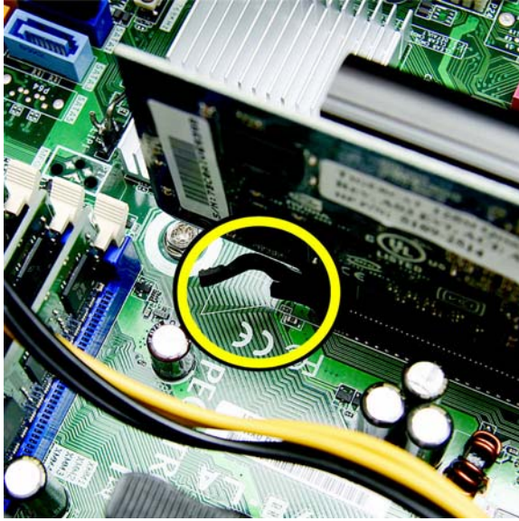
Figure 2-21 Replacing a graphics card
