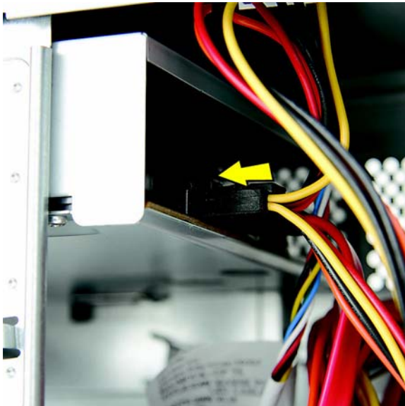
Figure 2-32 Connecting the power and data cables
