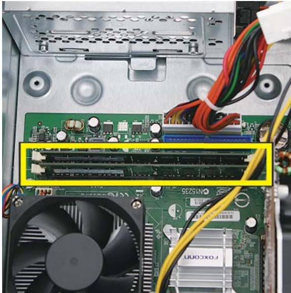
Figure 2-8 DIMM locations (500B shown)
