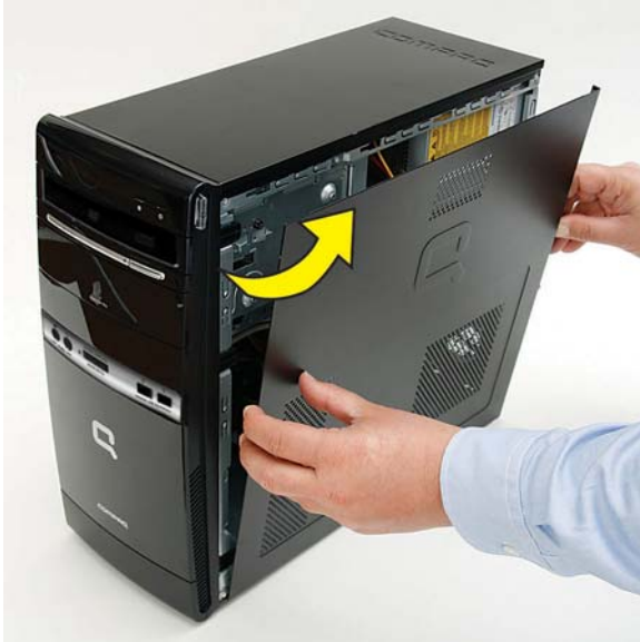
Figure 2-3 Removing the Computer Access Panel
