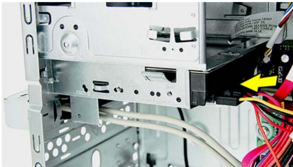
Figure 2-42 Attaching the connectors
