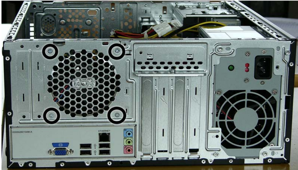
Figure 2-45 Removing the system fan
