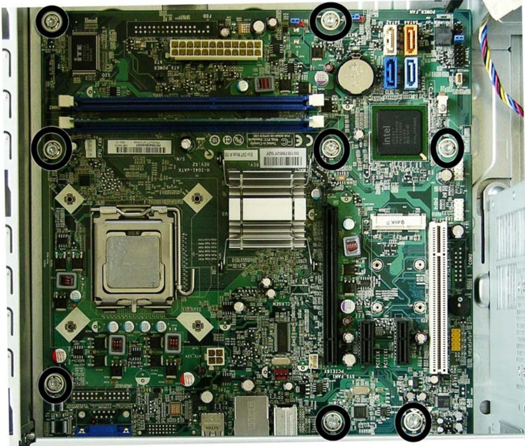
Figure 2-60 Removing the system board — model 500B shown
