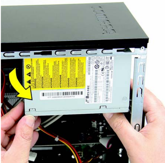
Figure 2-58 Removing the power supply from the computer
