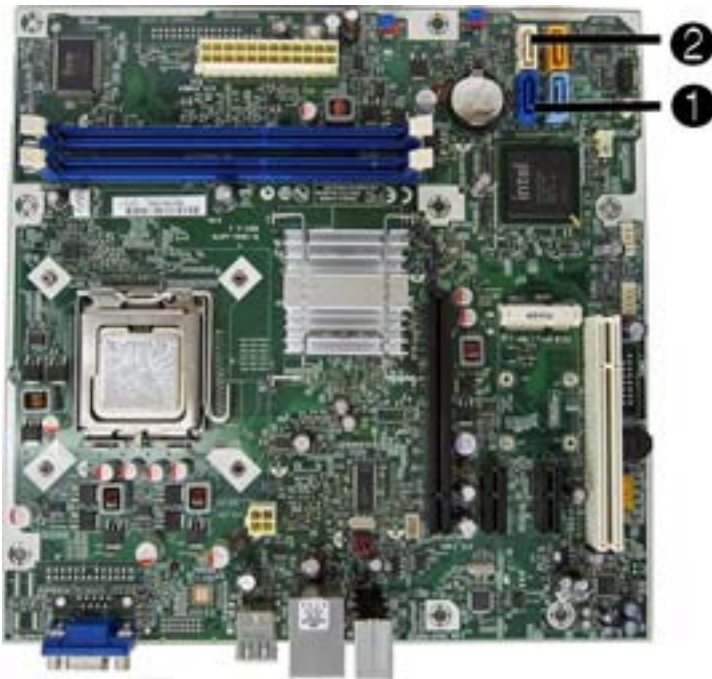
Figure 2-26 System Board Drive Connections — 505B/515B
