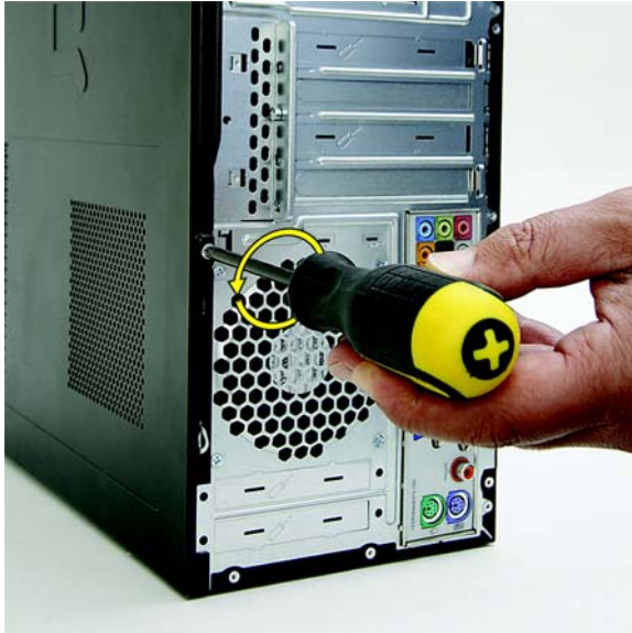
Figure 2-1 Removing the Computer Access Panel
