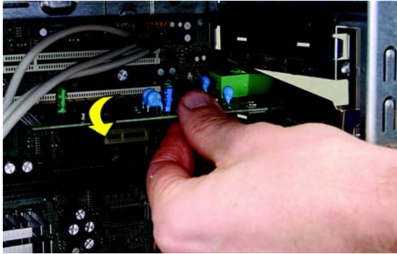
Figure 2-17 Rocking the card to Remove
