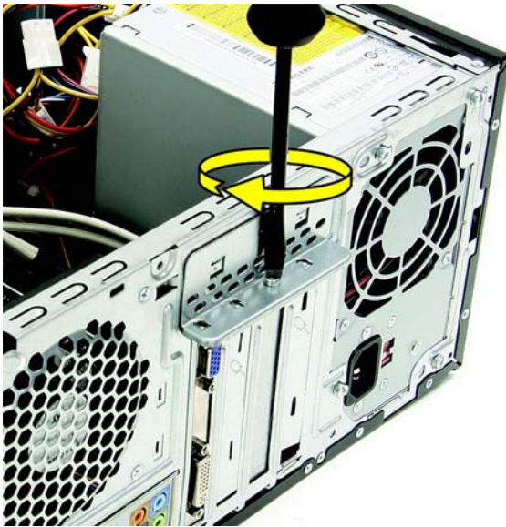
Figure 2-24 Replacing the bracket screw
