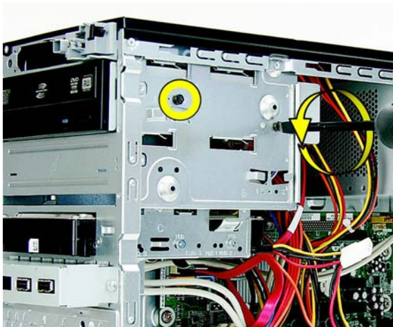
Figure 2-28 Removing the optical drive screws
