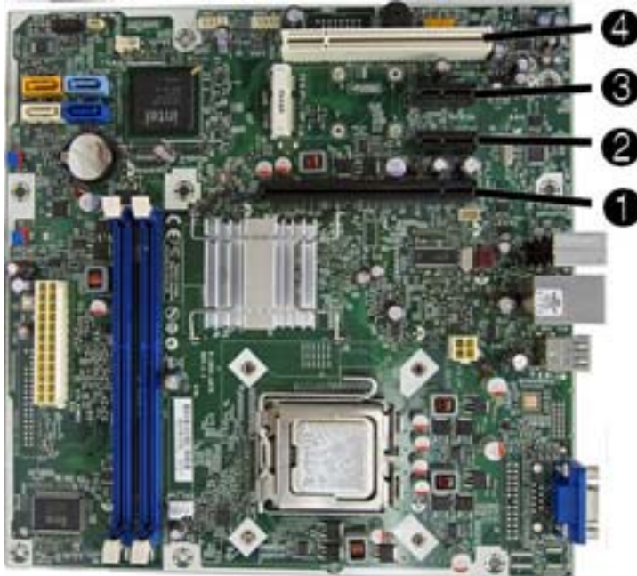
Figure 2-10 Expansion Slot Locations — 500B/510B
