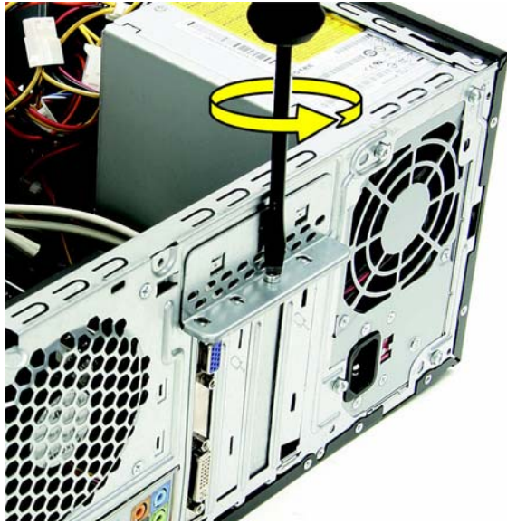
Figure 2-13 Opening the slot cover lock
