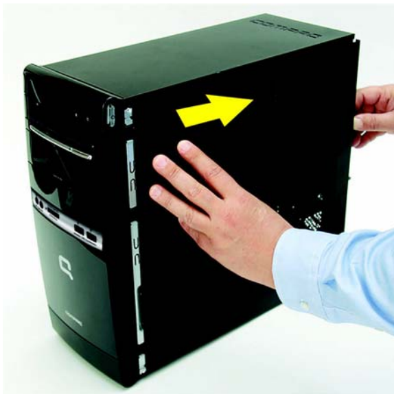
Figure 2-2 Removing the Computer Access Panel
