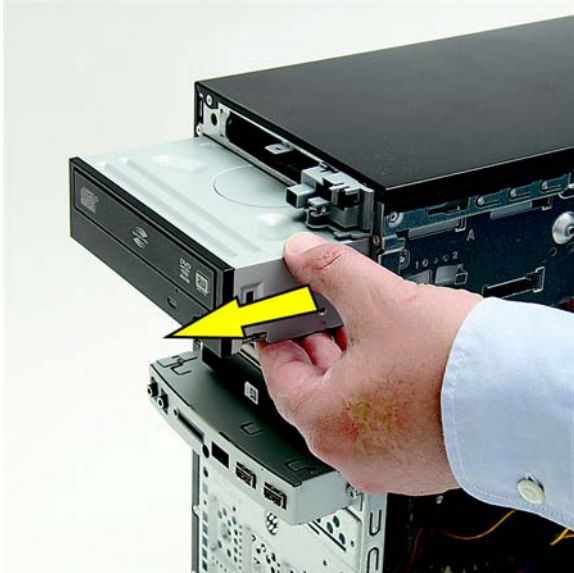
Figure 2-30 Pull the drive from the computer
