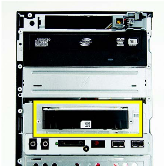
Figure 2-35 Locating the hard drive
