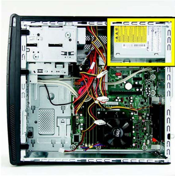
Figure 2-50 Locating the power supply
