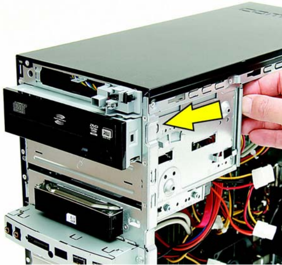
Figure 2-29 Push the drive forward
