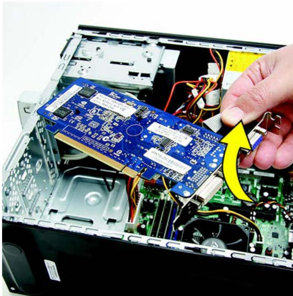
Figure 2-18 Lifting the card from the computer
