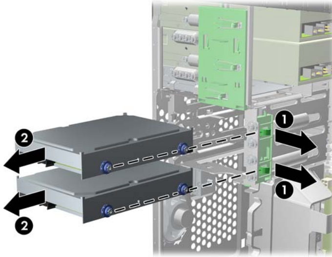
Figure 2-29 Removing a Hard Drive
