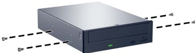
Figure 2-23 Installing Guide Screws (Optical Drive Shown)
