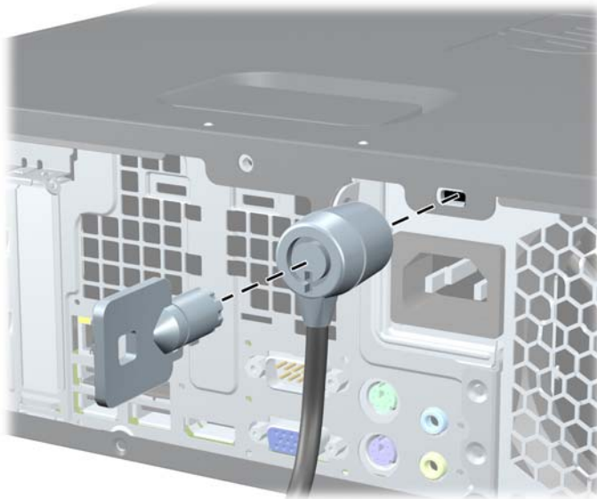
Figure C-1 Installing a Cable Lock
