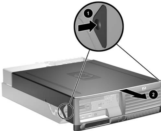
Figure 2-3 Removing the Computer Cover
