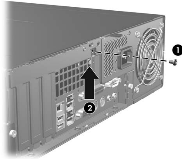
Figure 2-2 Removing the Smart Cover Lock Screw
