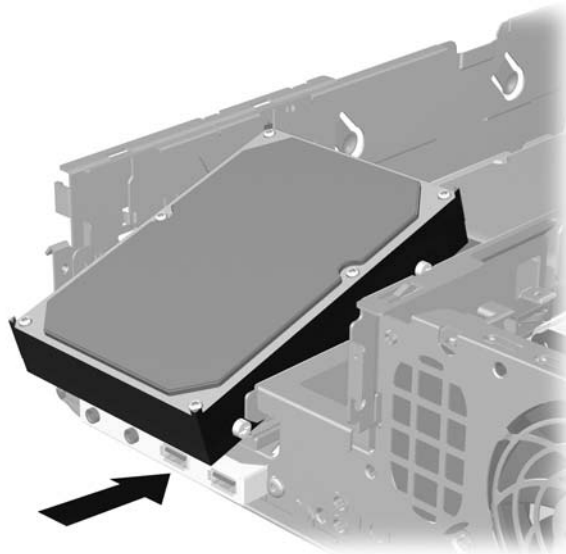
Figure 2-27 Installing a Drive into the 3.5-inch Drive Bay (Hard Drive shown)
