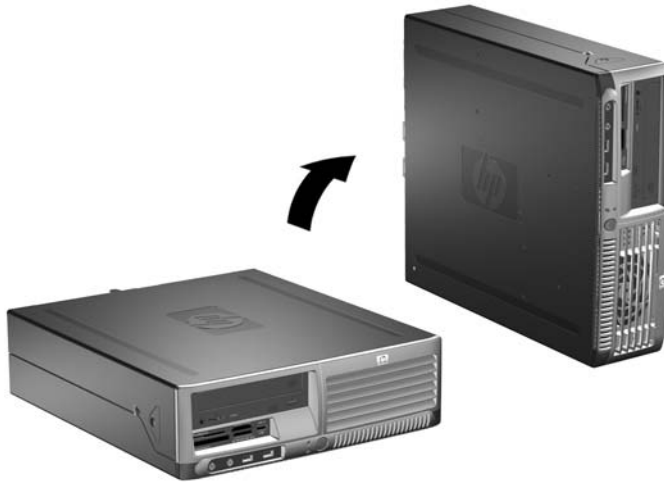
Figure 2-1 Changing from Desktop to Tower Orientation
