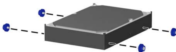
Figure 2-38 Installing Hard Drive Guide Screws
