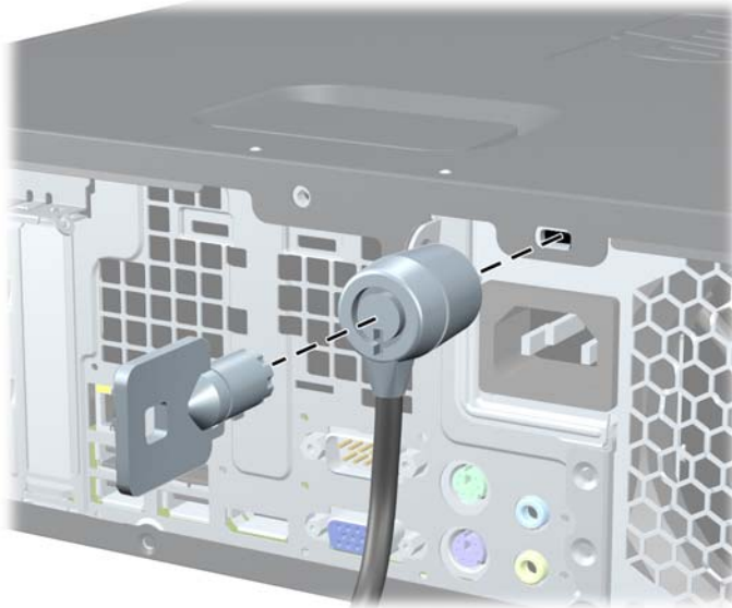
Figure C-1 Installing a Cable Lock
