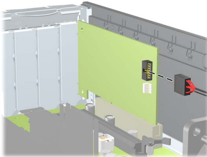
Figure 2-31 Disconnecting the Media Card Reader 1394 Cable
