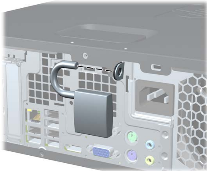
Figure C-2 Installing a Padlock
