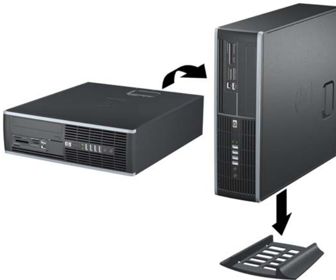
Figure 2-6 Changing from Desktop to Tower Orientation
