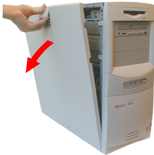
Shows how to remove the front panel
