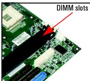
There are three 168-pin DIMM slots on the system board for installing main memory. You can install 133MHz SDRAM modules, these are available in 128, 256 and 512MB memory modules. 64MB memory modules are not supported. You can install a maximum of 1.5GB (3 x 512MB modules).
