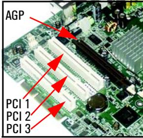
The XE320 has four accessory board slots: three PCI slots and one 1.5V AGP slot.
