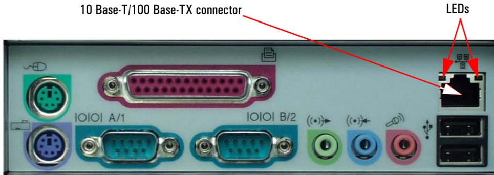
There are two LEDs on the 10 Base-T/100 Base-TX connector as indicated in the graphic above. The following table provides a status summary of these LEDs:
