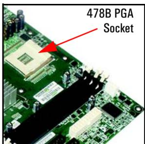
The XE320 is equipped with a socket 478B Intel Pentium 4 processor. The processor is connected to the system board through a Pin Grid Array (PGA) 478B Socket.
