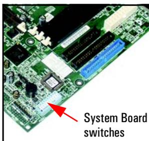
The following table gives the functionality and default position of switches on the system board switch block:
