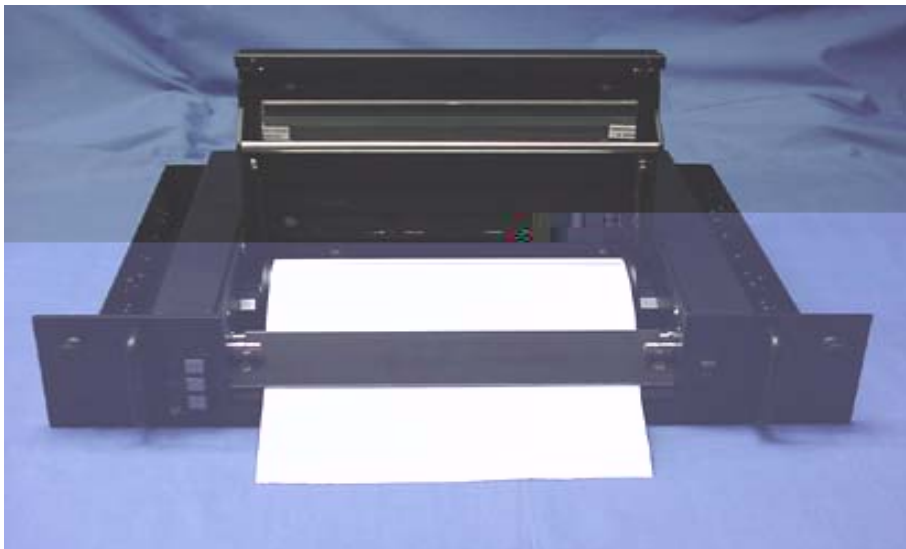
Figure 3-4 Roll paper installed
