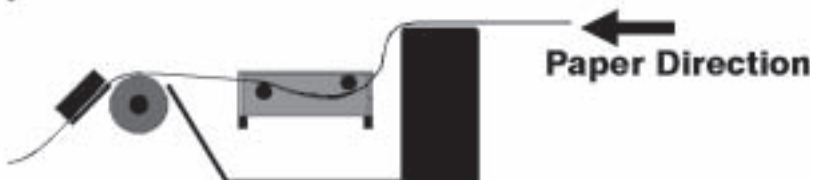
Figure 3- 7. Fanfold guide path
