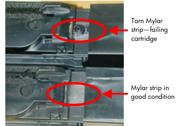
Print cartridge Mylar strip in poor and good condition
