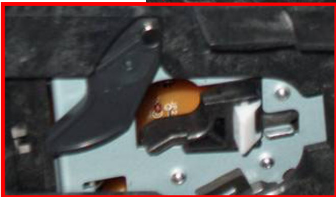
Location of cartridge alignment knob and detail
