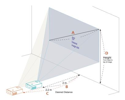
The table below shows how to achieve a desired image size by adjusting either the position or the zoom ring.
