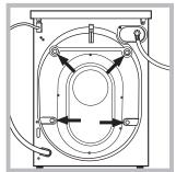
3. Remove the 4 protective screws and the rubber bush with the respective spacer, situated on the rear of the appliance (see also the installation leaflet).
