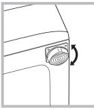
Install the washing machine on a flat sturdy floor, without resting it up against walls, furniture cabinets or other. 2. If the floor is not perfectly level, compensate for any unevenness by tightening or loosening the adjustable front feet (see figure); the angle of inclination, measured according to the worktop, must not exceed 2°.
